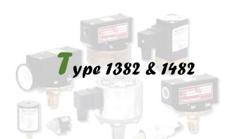
This series of pressure switches are used to monitor the difference between two pressures. For example, they can be used to monitor filter condition and signal when the filter is becoming blocked. They can also be used as flow monitoring switches if used across orifice plates etc.
