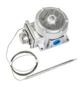
nVent RAYCHEM Raystat-EX-02 is a hazardous area mechanical surface sensing thermostat providing temperature control for heating cables. Switching temperature range -4 °C to 163 °C, adjustable externally to the Ex enclosure by a dial mounted under a bolted-on cover and seal. Switching current capacity is 22 A.
