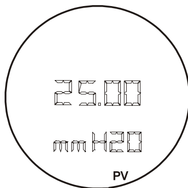
Fig. 2.5 – Typical Monitoring Mode Display Showing PV, in this case 25.00 mmH 2 O
